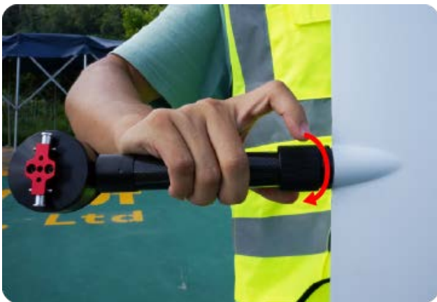
Installing the elevator
