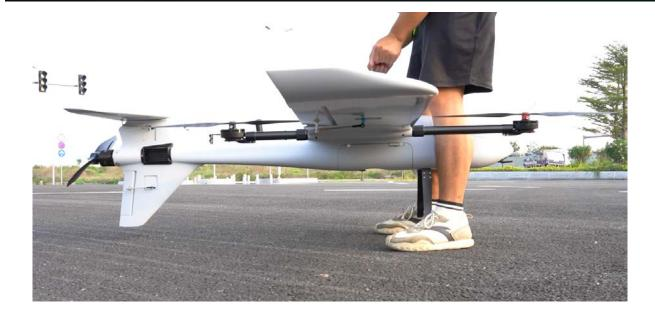
**Note:** The position of the center of gravity will affect the flight stability and flight efficiency. Before flying, it is necessary to confirm the balance of the center of gravity
