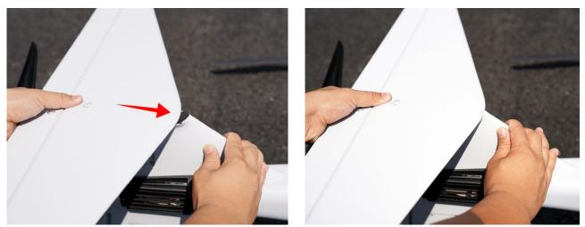
Pull the quick-release lever to protrude from the slot, and then install it into the ball head.
