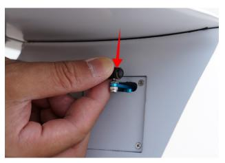
Hand-tighten the screws into the tailfin and ensure they are secure.
