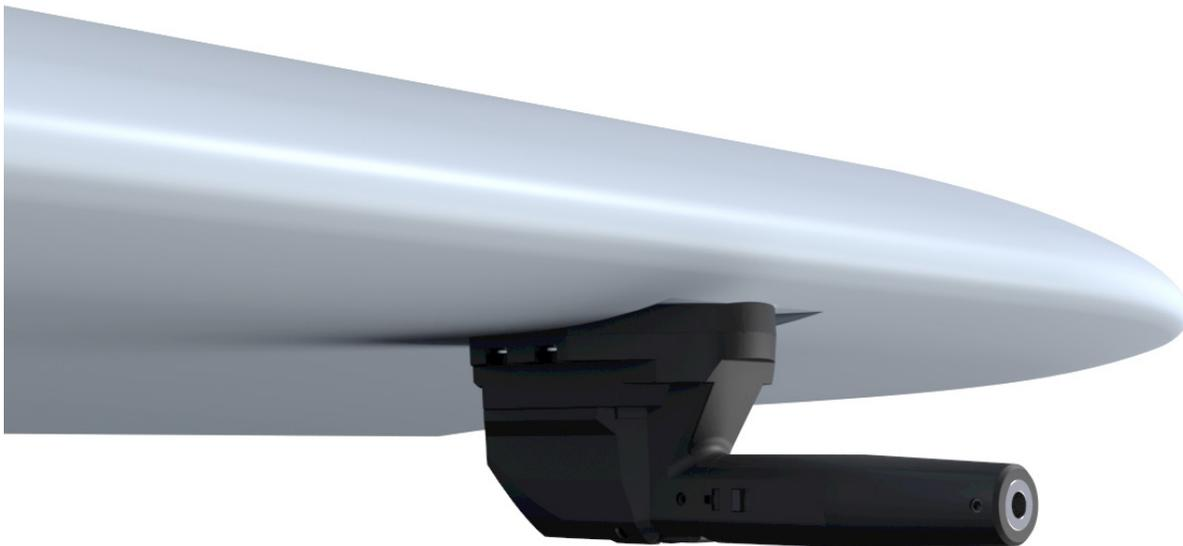
Note: The rotation of the propeller will cause airflow disturbance, which will make the UAV obtain wrong airspeed data. It is forbidden to install the airspeed near the propeller.
